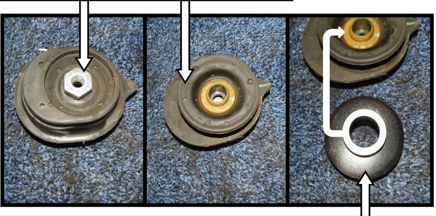
🇬🇧 Install V-Maxx spring seat to original top-mount and bearing
