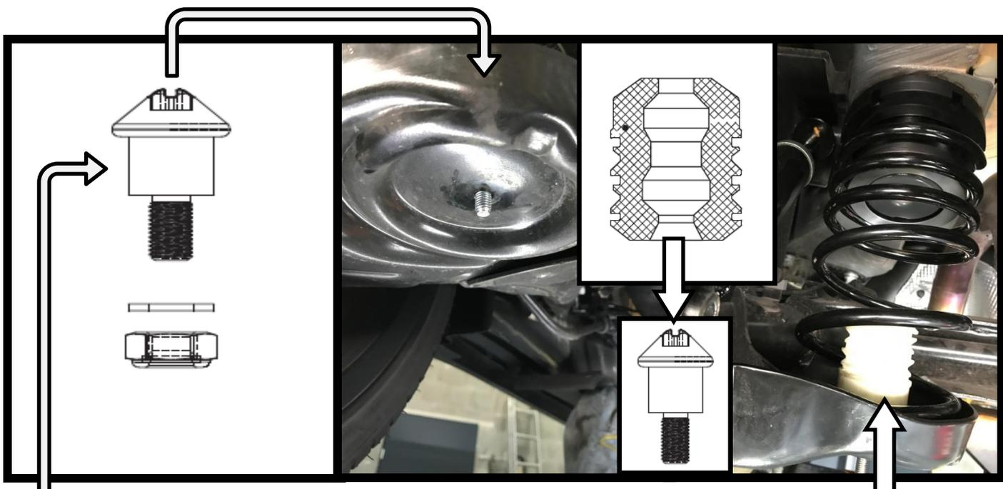
🇬🇧 Install the supplied special M8 bolt to bottom of the rear axle , and slide the supplied bumpstop over the top of the special bolt.
