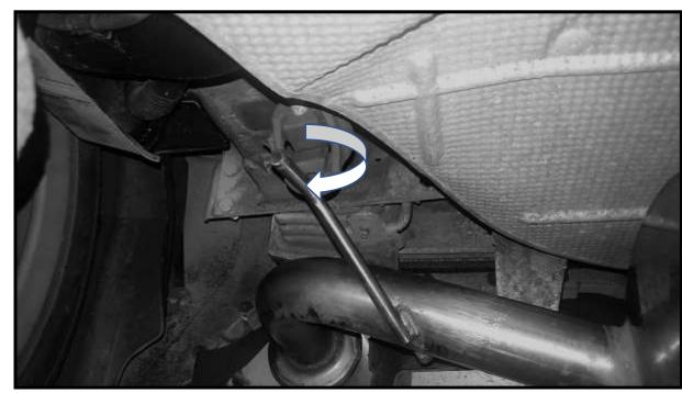
7. Connect the plug to the electric valve and secure the wires with the strap so they do not touch the exhaust pipe.
