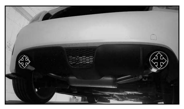
9. Once the exhaust is aligned, tighten the connection with the clamp.
