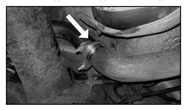
5. Place the exhaust brackets on the rubber hangers
